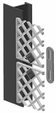
Isometric view of ANC H-Posts, Panels, Wedge Plugs and Back Straps
